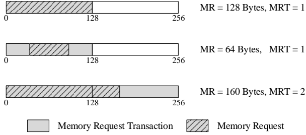
Fig. 2. Examples of the relations between Memory Requests (MR) and the needed Memory Request Transactions (MRT). All the three examples apply to DMA while only the middle one applies to Gload, because Gload can only request up to 32 bytes.
