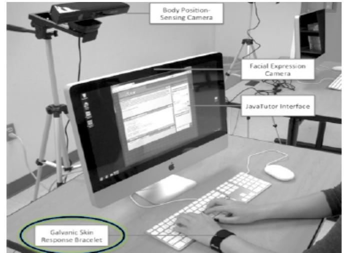
Figure 1. Study Setup. Skin conductance data measured through a Skin Conductance Bracelet.
